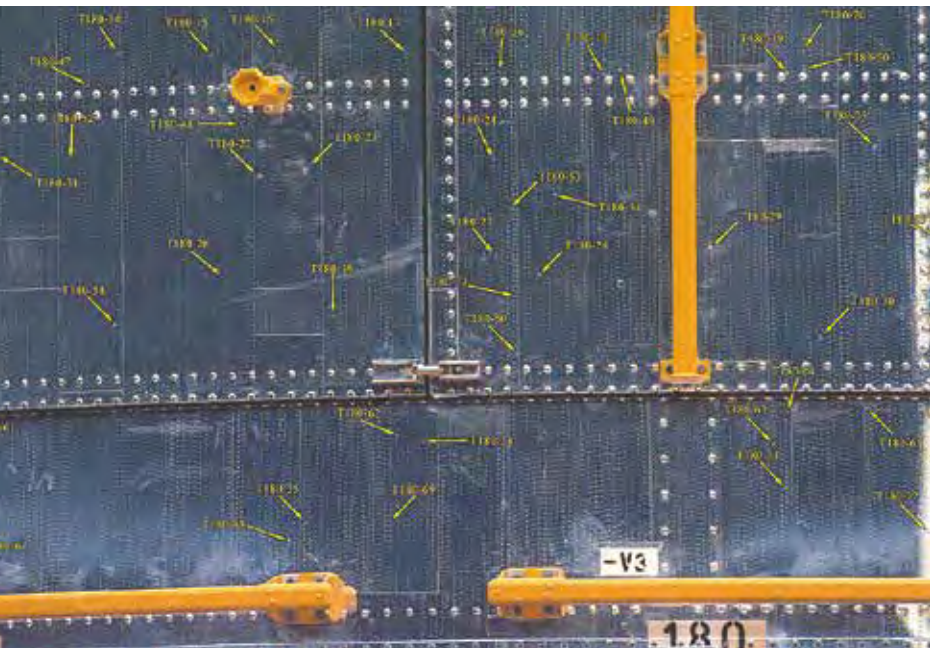
This part was removed from the Hubble Space Telescope during in-space repairs. The yellow arrows show the damage from many orbital debris impacts.
